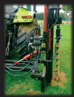
The Rock Spike Extractor System (RSE), can be used with a spike, an auger, or both.
