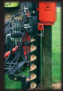
The auger swings back into the transport position so you can drive the post into the hole.
