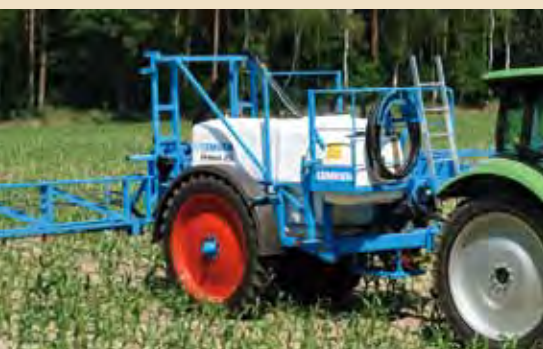
Close coupling ensures sprayer wheels follow tractor wheels as closely as possible
