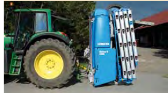
Quick attachment using the QuickConnect system
