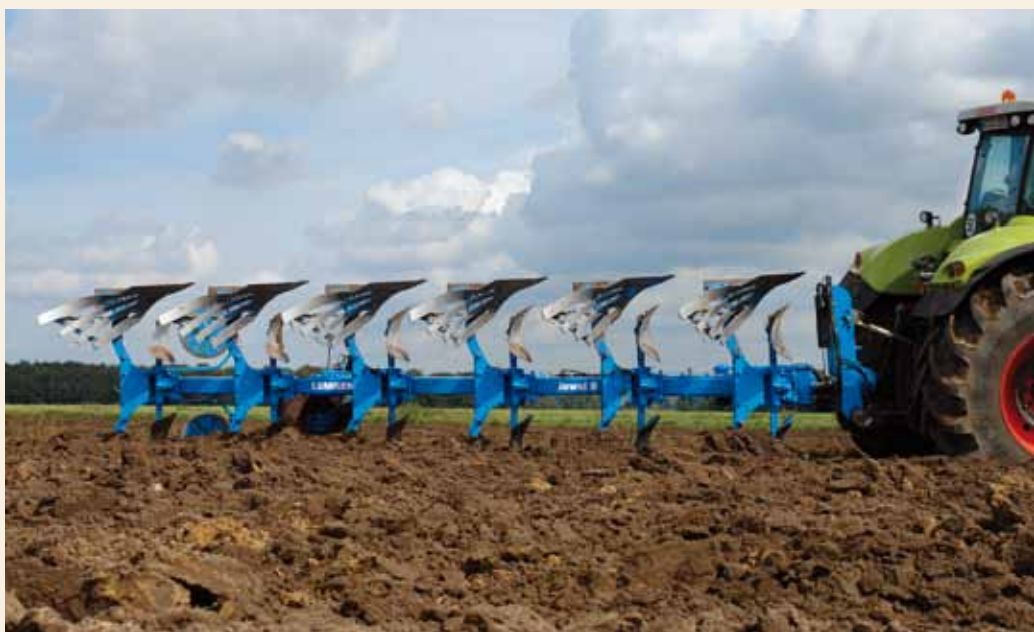
The OF version, of the new Juwel mounted plough, is suitable for ploughing both “in the furrow” as well as “on-land”.
