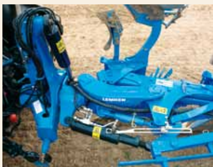
The completely new electro-hydraulic turnover device allows simple and efficient adjustment of pitch without leaving the cab.
