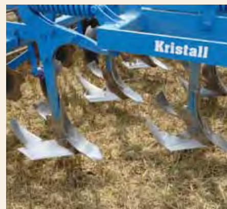
The new Kristall cultivator with 7 tines (left) compared with the Karat cultivator with 11 tines. Working width is 3 m in both cases.
