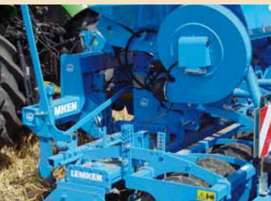
The hydraulically driven fan
