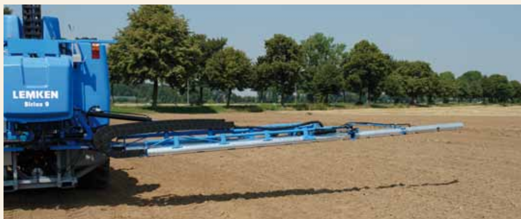
The outer section 4, with lateral break-back, is folded down and sections 2 and 3 retracted to give a narrow spraying width.
