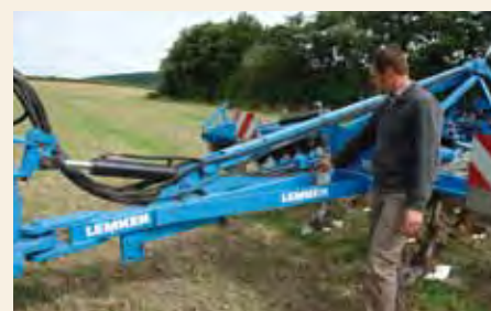
The hydraulic traction assistance can be activated by opening a tap
