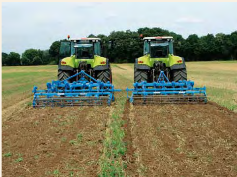
The new Kristall cultivator with 7 tines (left) compared with the Karat cultivator with 11 tines. Working width is 3 m in both cases.
