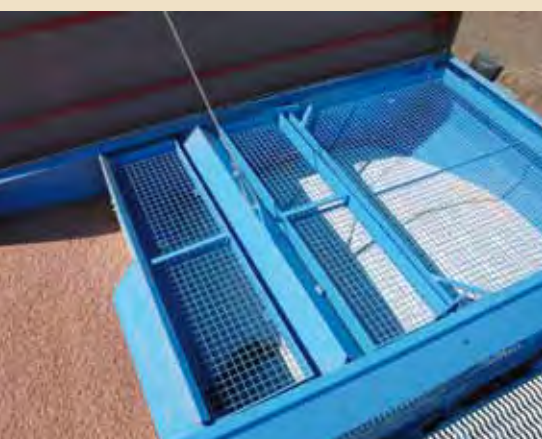
The divided hopper on the Compact-Solitair HD
