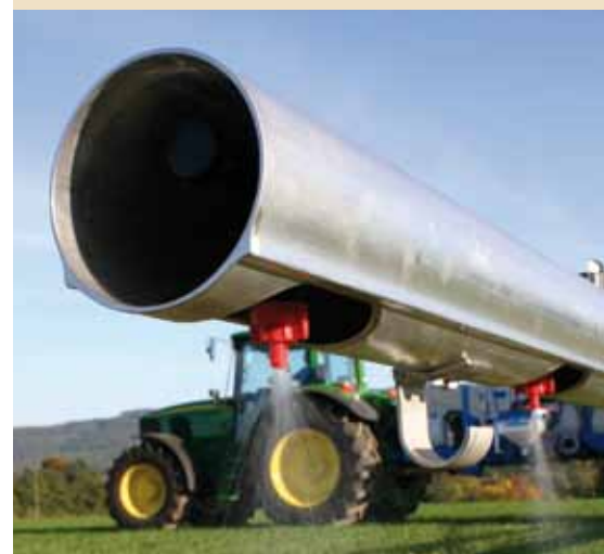
Proven design: Boom made from aluminium tubing
