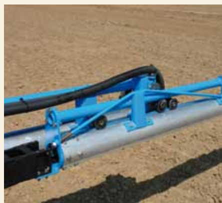
With VariExtend, boom sections slide past each giving an infinitely variable working width.
