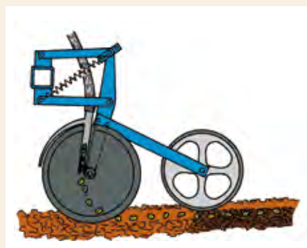
Parallelogram-mounted Double Disc coulters
