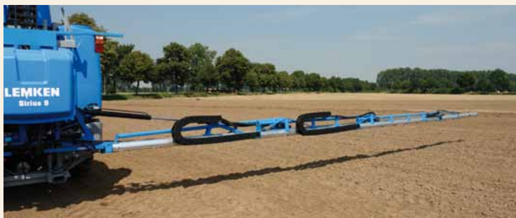
The outer section 4, with lateral break-back, is folded down and sections 2 and 3 extended to provide maximum spraying width.
