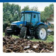
Matched forward and reverse speeds The 20x12 Synchro Shuttle™ transmission features a synchromesh reverse lever. Changing direction is fast and easy, with matched forward and reverse speeds. This enables turns to be made faster at the end of the field or when working with a front loader.
