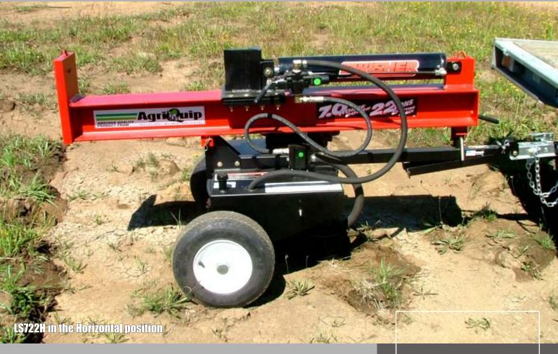
Whether you prefer splitting wood vertically or horizontally - here's the answer - a splitter with both options ready for action by removing a pin. A fully independent splitter with it's own 7HP engine and hydraulic system. Fully transportable and simple to operate.
