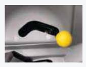
On Synchro Shuttle™ cab models, the PTO is positively engaged courtesy of an ergonomically positioned servo-assisted lever for effortless actuation.
