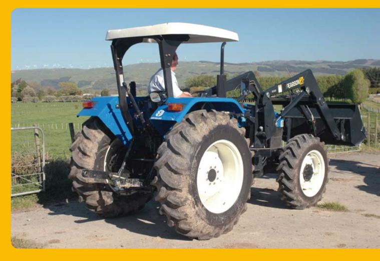
The two model TT Series are supplied with a 2-post ROPS factory designed canopy. Standard specification includes eight forward and two reverse speeds and an independent PTO system. Available with a front end loader, this enables an extensive range of different applications to be carried out and ensures a TT Series tractor meets every operators' requirements.
