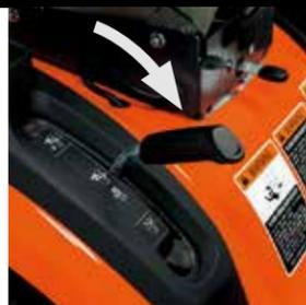
**3** Release the lever to lower the deck
