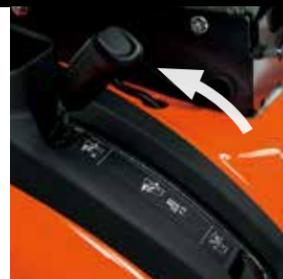
**1** Pull the lever to lift the deck
