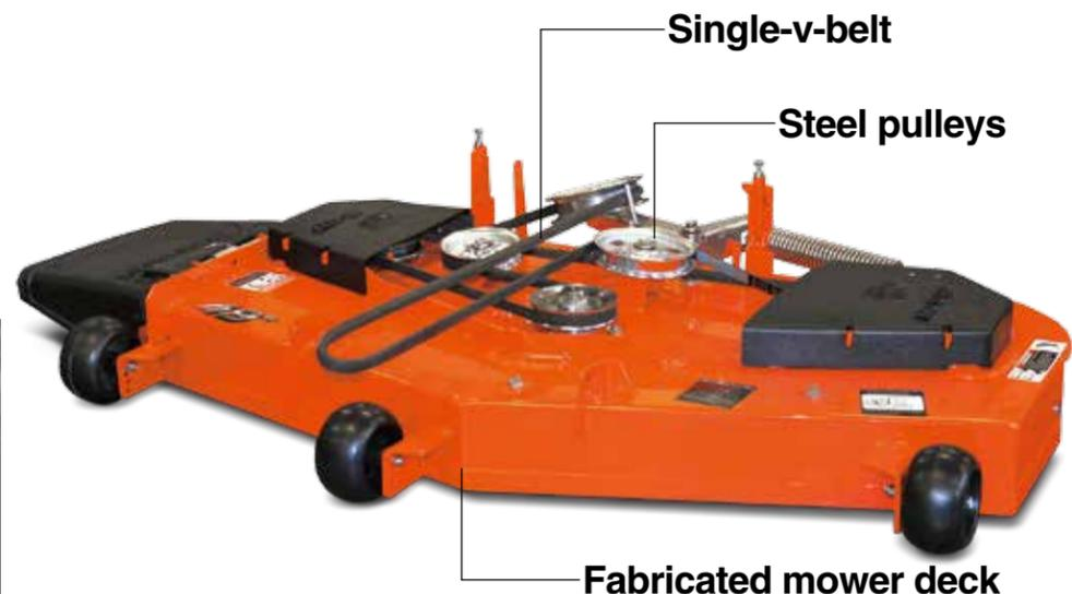
Fabricated mower deck
