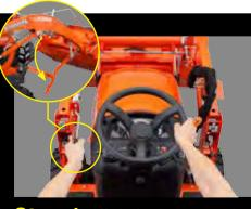
Step 1: Lift the loader boom and fully dump the bucket.
