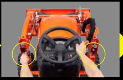
Step 2: Unlatch the loader latch levers to detach the front loader hooks.
