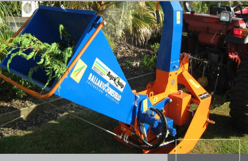
The Agriquip BF100 PTO driven chipper shredder features a unique combination of a chipper blade and shredder knives that will efficiently chip and shred hard and green vegetation.
