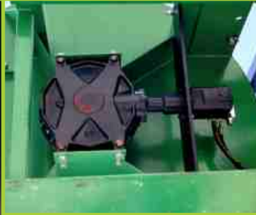
hydraulic drive on DBM750 (option)
