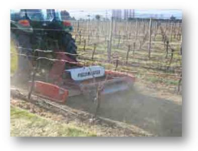
Fieldmaster developed this concept because of market concerns expressed about flail drum mulchers, specifically; very slow ground speed, expensive running costs, expensive maintenance bills – particularly downstream parts and service costs associated with rebalancing misaligned drum rotors.
