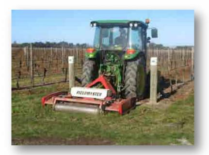
By simply changing blade systems, Fieldmaster multicut rotary Gearmowers are transformed into a fast, effective rotary mulcher. This does away with need for a second slow, inefficient and expensive flail drum mulcher.
