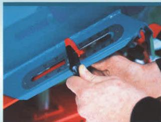
Precise rate adjustment on stainless steel graduated quadrants
