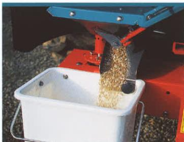
The rate calibration kit : a recommended option by SULKY when looking at controlled fertilising techniques.
