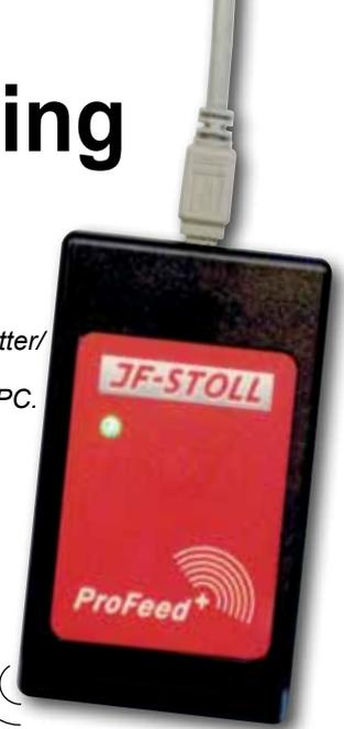
Wireless transmission of data between main terminal in the loader and the PC in the office.
