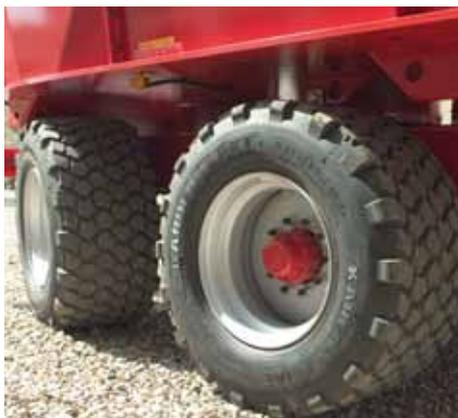
Spring-loaded bogie, fixed or turnable rear axle. VM 22-2 B has 1 axle as standard.
