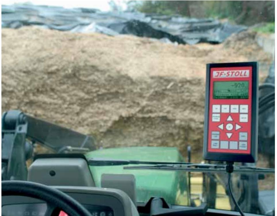
The JF-STOLL Feeder has wireless display as standard. With the display placed in the loading tractor great flexibility is achieved during loading. This is time-saving, gives an maximum comfort and minimises the feed loss.
