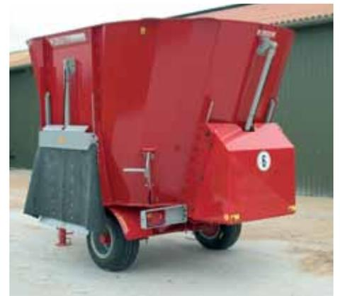
Example of a VM 10-1 which has been fitted with an additional rear door due to the barn arrangements.
