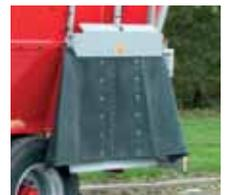
Discharge doors with rubber/steel guard
