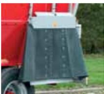
Discharge doors with rubber/steel guard
