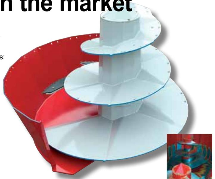
JF-STOLL is the first producer of complete diet mixers who has taken the step and introduced high strength steel S500/650 in the production of diet mixers. The use of high strength steel is especially important in connection with the auger windings and the first 50 cm of the tub walls, which are the parts that are exposed to the hardest wear.
