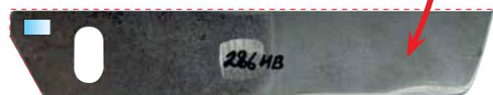
High strength steel (S650) after the test
