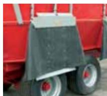
Discharge doors with rubber/steel guard
