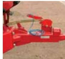
Overrun brake (Germany) with brake lock when reversing.
