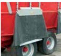
Discharge doors with rubber/steel guard
