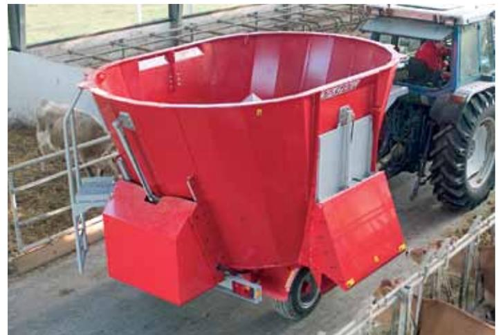
The strong steel guard opens immediately when operating the door. The large opening gives free passage for the feed.
