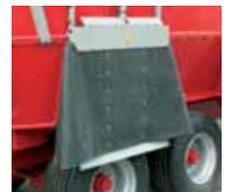
Discharge doors with rubber/steel guard
