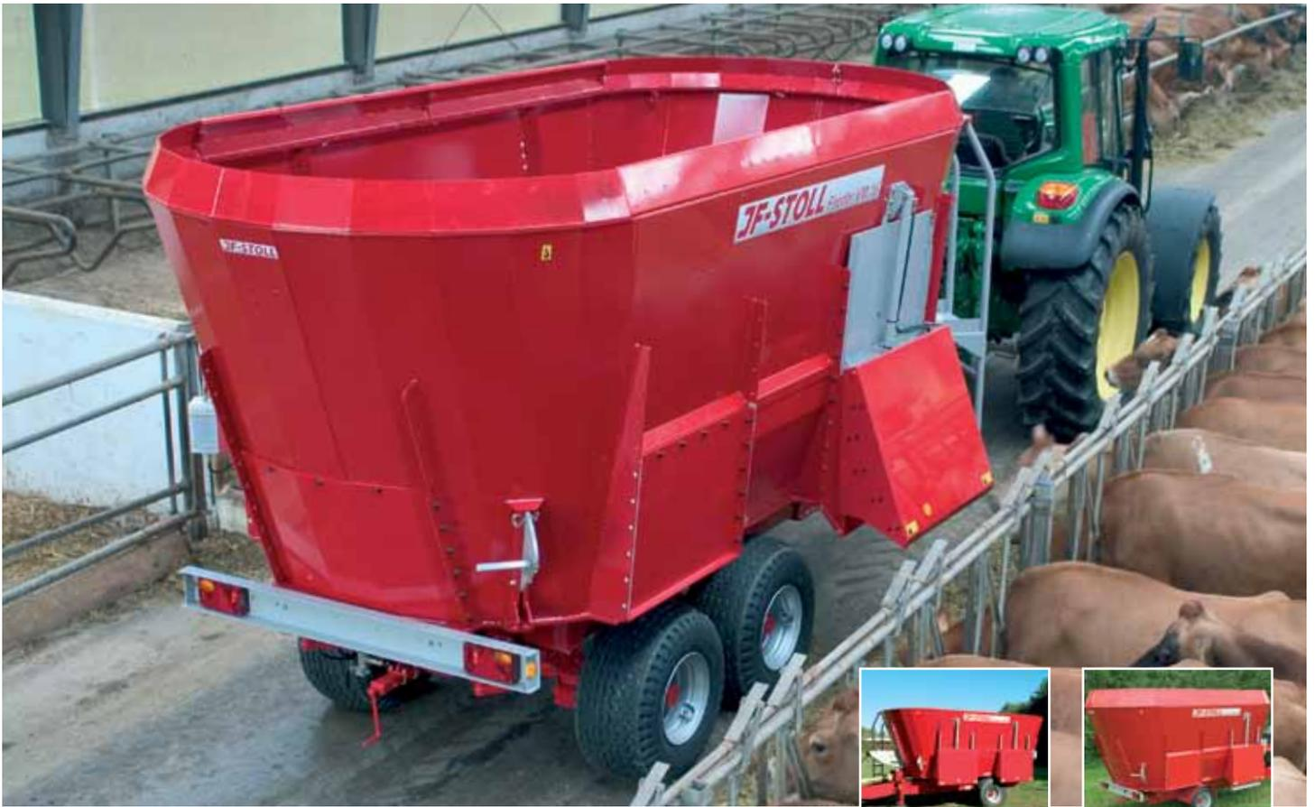
VM 16-2 S mounted with spring-loaded bogie and pneumatic brakes
