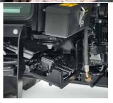
**MID MOUNT REMOTE VALVES** The T4 PowerStar range is specified with two mechanical mid-mount remote valves to operate mid mounted equipment or a loader. They are controlled via an ergonomic, fully integrated joystick in the cab.
