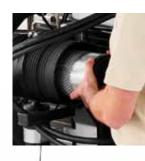
The engine air filter is easy to check, clean or replace, with no need for tools.
