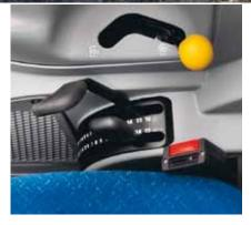
**MECHANICAL DRAFT CONTROL** Mechanical draft control offers proven reliability when returning an implement to work during a headland turn sequence and maintains a constant draft load. This simple, easy to operate system uses dedicated controls located to the right of the operator.
