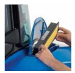
Replace or clean the cab air filter by simply removing from the easy access fendermounted position.
