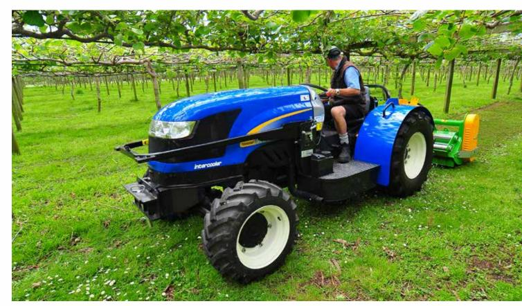
Tailored range of orchard tractors to suit pergola grown kiwifruit or where low operating heights are required, available in 65, 78 and 88 horsepower. The end result is a low profile orchard tractor, with great ground clearance, that offers a very good power to weight ratio with the right wheel equipment to utilise it. Getting on and off this tractor is a breeze.
