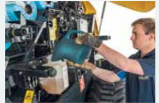
Chains lubricated with universal 10-40 oil. Chain oiling brushes operate each time the baler tailgate is opened.
