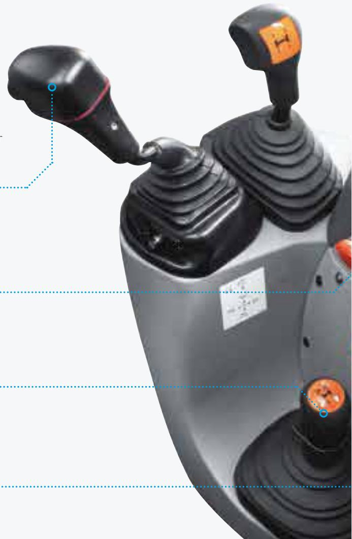
The mechanical joystick controls up to four mid-mount remotes, ideal for operating a front loader with ease from the comfort of the driver's seat.
